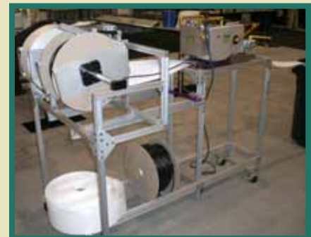
Adjustable Guide System for Various Cord/Flap/Seam Sizes
