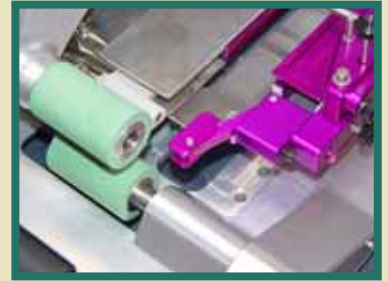
Flat Hem Pressure Arm and 2" Pressure Rollers
